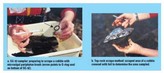
**Figure 7.2.** How to remove algae from rock surface and how to measure rock surface area. (USGS 2002.)
