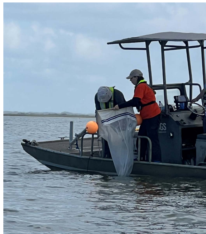
FIGURE 3.13 Collecting microplastics with a net towed by a boat (Photo by GBEP)
